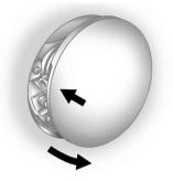
The tethered fuel cap is located behind a hinged fuel door on the passenger side of the vehicle.
